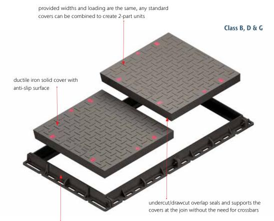
frame fits around both covers without the need for additional support, the undercut/drawcut profile supports covers across the middle
