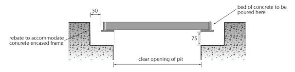
Due to the varying frame dimensions for different covers and decorative edging options, dimensions shown indicate the minimum amount of concrete required around the frame. Full details at www.acoaccess.com.au/ product-support/installation-guidance/ Concrete of a minimum strength of 32MPa and minimum aggregate of 12mm is recommended.
